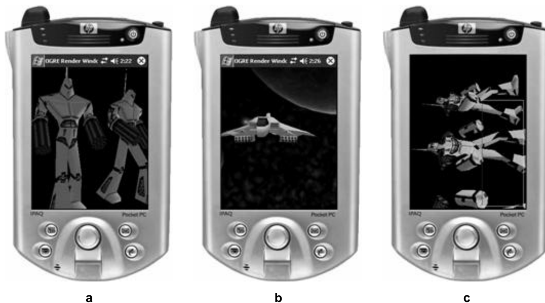
Figure 2. Screenshots of OGRE demos on Pocket PC: a) SkeletalAnimation using OpenGL ES RenderSystem b) SkyBox using OpenGL ES RenderSystem c) SkeletalAnimation using Klimt RenderSystem
